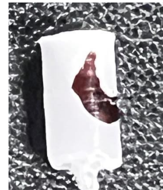
Degraded material from granulation process at polymer supplier (rare)
